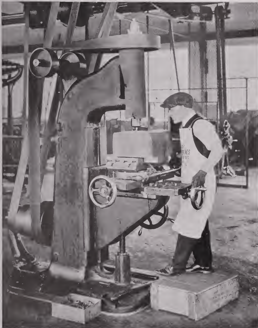
PRATT & WHITNEY PROFILER One of a Battery of Three.
